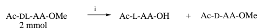
Scheme 1 Enantioselective, pronase catalysed hydrolysis of racemic N -acetylamino acid esters (Ac = acetyl, AA = amino acid). Reagents and conditions: i, 20 mg pronase, 2 cm 3 THF, 20 cm 3 phosphate buffer (pH 7.0, 0.067 mol dm -3 ), room temp.
